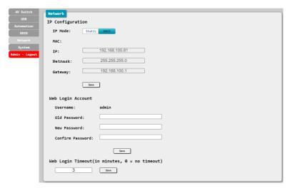
1) IP Configuration: IP Mode may be switched between Static IP or DHCP. In Static IP Mode the IP, netmask and gateway addresses must be manually set. When in DHCP Mode, the unit will attempt to connect to a local DHCP server and obtain IP, netmask and gateway addresses automatically. Please press "Save" after making any changes to the IP configuration or mode.
